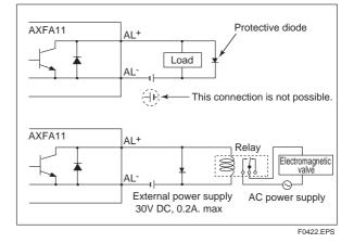
Figure 4.4.14 Alarm Output Connection
